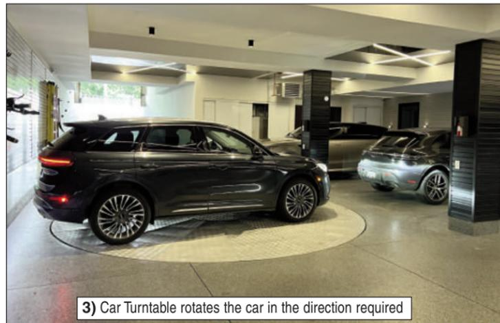
3) Car Turntable rotates the car in the direction required
