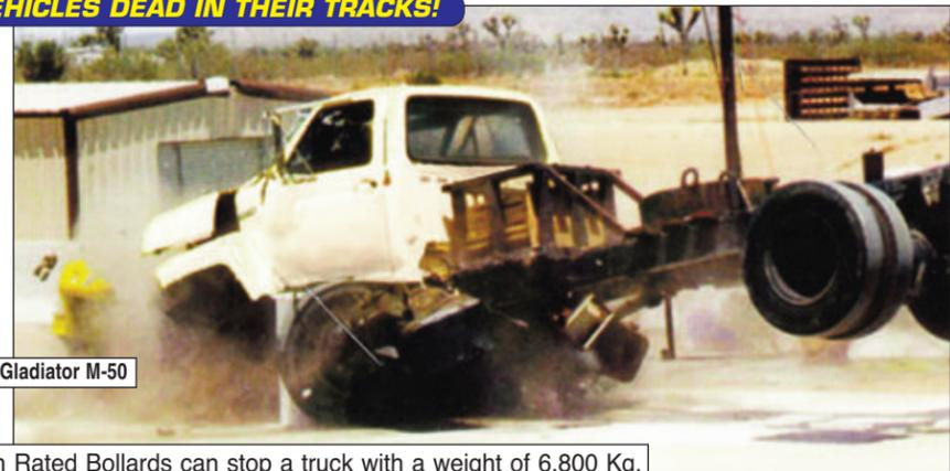
Superior Crash Rated Bollards can stop a truck with a weight of 6,800 Kg. going 80 Kph dead in its tracks with a maximum penetration of 1m.
